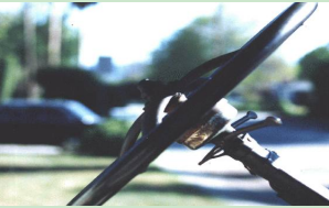
The throttle was worked by hand on the T. Note the large -- and lethal -- bolt topping the steering column.
